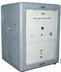
The first-known SAR 11-bit ADC is built by Bernard Gordon at EPSCO. It was based on vacuum tubes.
