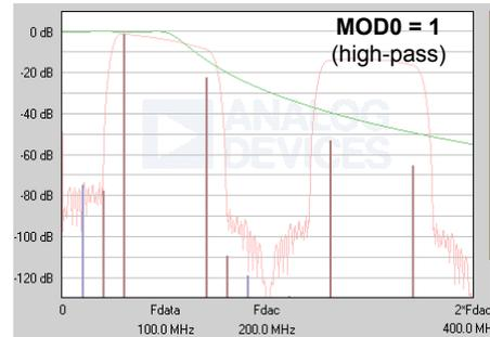
The AD9772 also has a "zero-stuffing" mode (↓ **MOD1 = 1**) which allows the data stream to be doubled a
