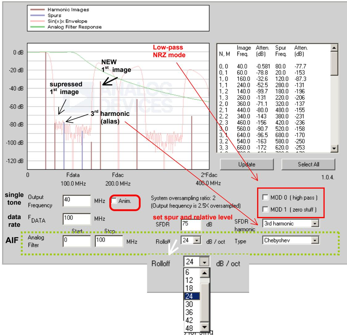
The model of the [AD9772A](#) is simplified and idealized - only SFDR is modeled and it is assumed frequency-independent. The AD9772A contains an integral **interpolator** which *doubles* the input data rate. The interpolation filter suppresses the upper image in **low-pass** mode (**MOD0 = 0**), or suppresses the fundamental when in **high-pass** mode (**MOD0 = 1**). The response characteristics of the internal digital filter have been approximated.
