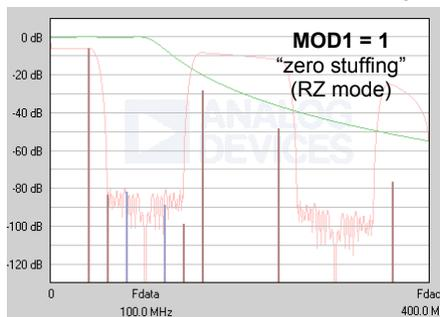
second time by inserting zeroes between each sample. Zero-stuffing doubles again the number of images per  $F_{DAC}$  harmonic, but  $F_{DAC}$  is twice what it would be without zero-stuffing and the mathematics work so that the location of the images is the same as without zero-stuffing - only the amplitudes change. These new images are not filtered internally so that the upper image can be used for direct IF synthesis. MOD0 and MOD1 are often used together for this purpose.
