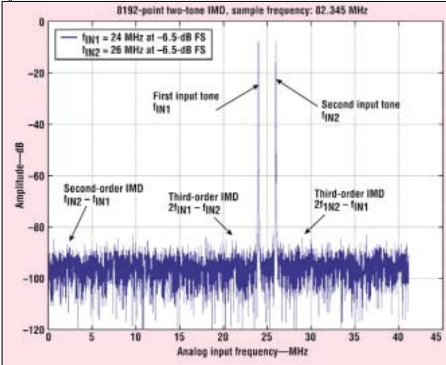
2. The two-tone intermodulation distortion for the MAX1448 was plotted with a sample frequency ( $f_{\text{SAMPLE}}$ ) of 82.345 MHz.
