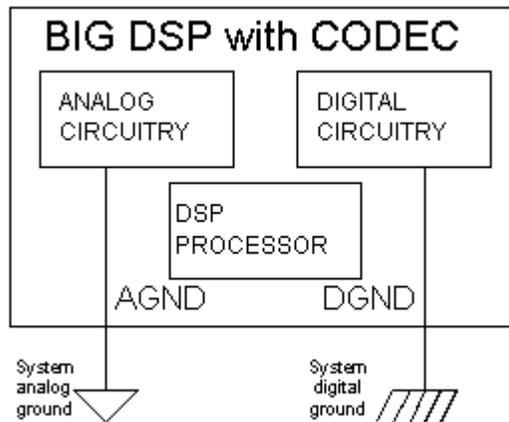
The only **exception** which the Applications Department at Analog Devices has yet discovered is big DSP processors which happen to contain codecs. These devices draw hundreds of mA of transient current in their DGND pin, and are also designed so that noise on this pin does not feed to their analog/converter circuitry. They are best used with their AGND pin to analog system ground and their DGND pin to digital, unless their designer suggests otherwise.
