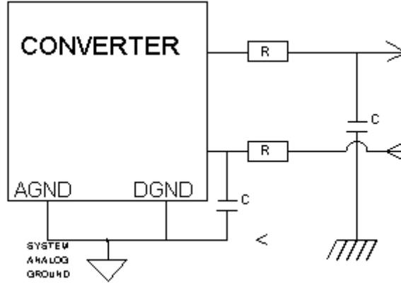
Noise feedthrough can sometimes be reduced by slowing the edges of digital signals going to and from a converter. This may be done with an RC network. But this also increases propagation delay and may disrupt system timing. It is a useful technique but must be used with caution and possible ill effects carefully analysed.
