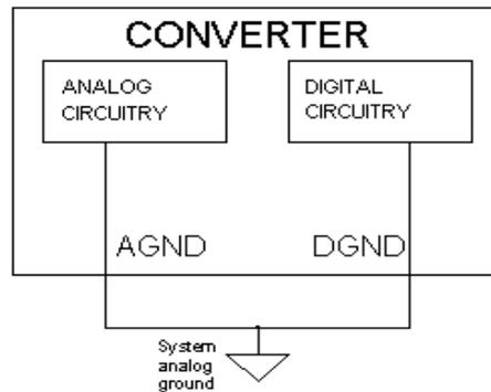
This, of course, raises the question of why a pin designated "Digital Ground" should be connected to the analog ground of the system.
