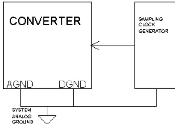
Phase noise in sampling and reconstruction clocks can devastate the performance of a sampled data system. This is, in fact, the subject of a separate lecture in this series. One way to minimise phase jitter is to ground the sampling clock generator to the system analog ground, so that the converter and the clock share the same ground, and common-mode noise between grounds does not phase modulate the clock signal
