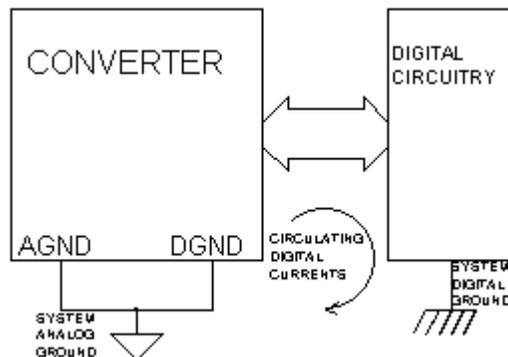
With proper decoupling the only digital currents to flow between the system analog and digital grounds are the return currents of the converter's logic interfaces. These should be kept as low as possible.
