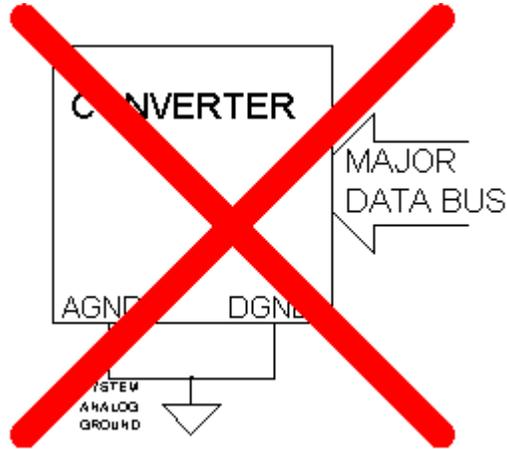
It is important never to drive a data bus directly from an A-to-D's parallel port - the digital currents are likely to be too large. In addition to the ground return current problem we have mentioned, large output currents from a converter increase its dissipation - which may affect its accuracy due to thermal effects. DACs also suffer from this type of connection - bus noise corrupts their analog output
