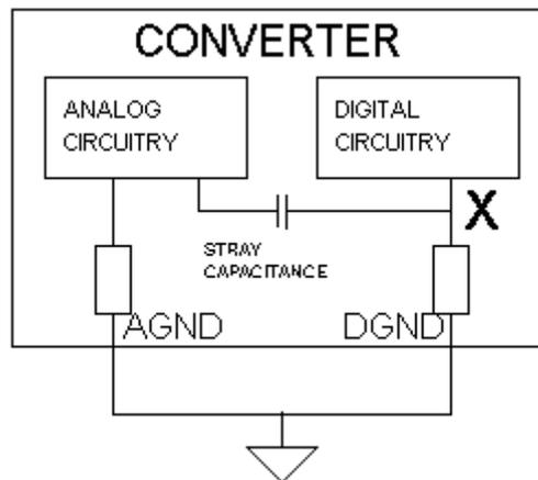
Noise in its digital circuitry can couple to the analog part of the converter by stray capacitance. Ground noise coupling is minimised if the noise voltage at node X in the diagram is as small as possible.
