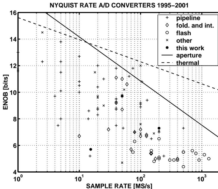
Figure 2.6 High-speed A/D converters from years 1995–2001.
