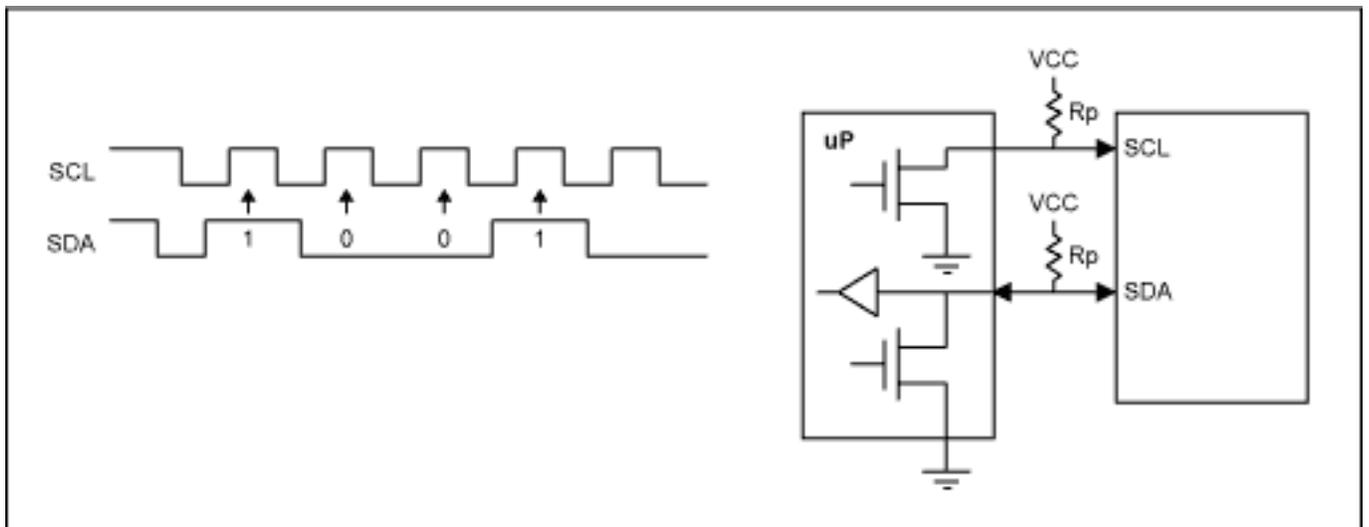
Figure 2. Signals and timing of the I<sup>2</sup>C-interface
