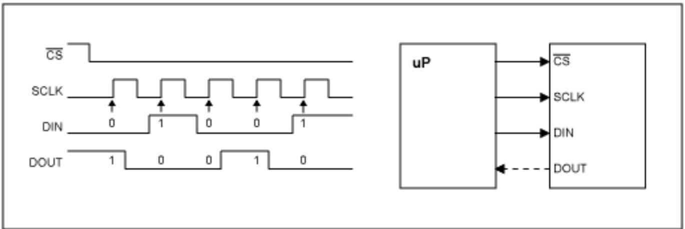
Figure 1. Signals and timing of the SPI-interface
