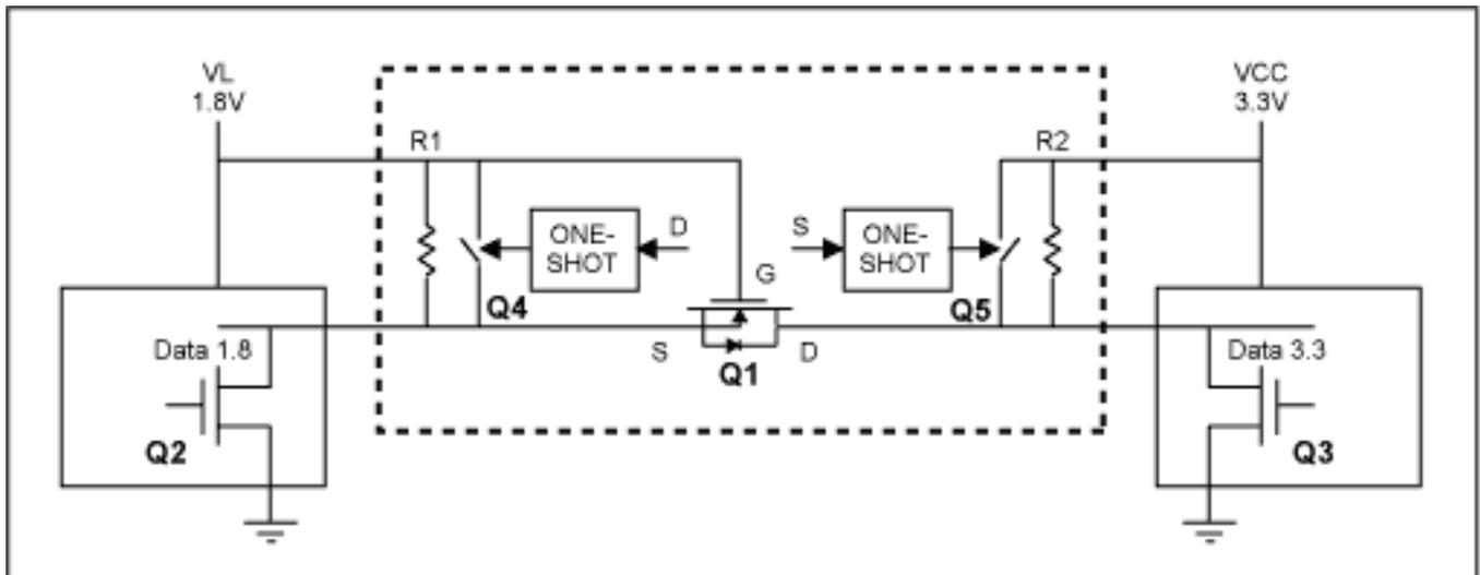
Figure 4. Improved level translator MAX3373E with speed-up circuit
