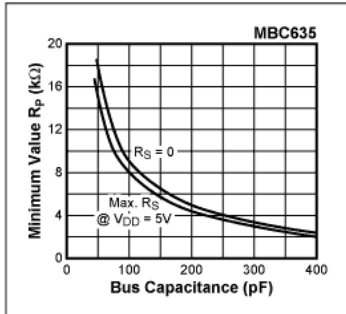
Figure 8. Minimum value of  $R_p$  as a function of supply voltage with the value of  $R_s$  as a parameter, from I<sup>2</sup>C-specification
