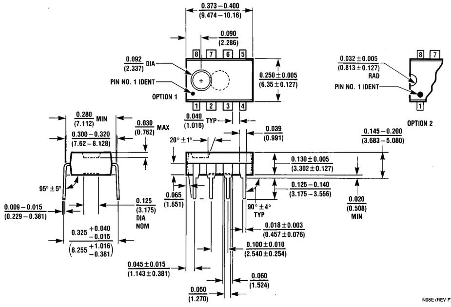
**8-Lead (0.300" Wide) Molded Dual-In-Line Package**
