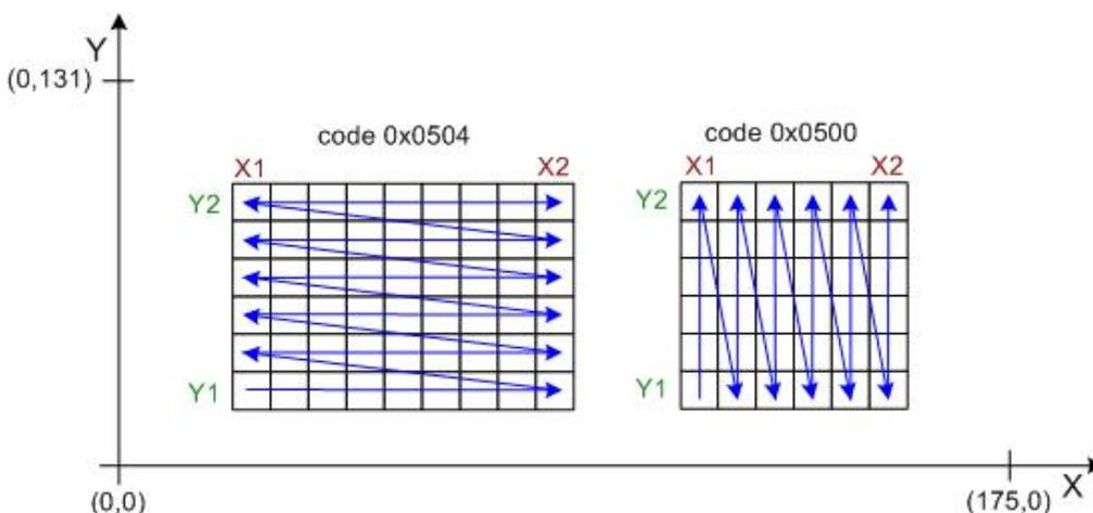
For partial writing to the memory the commands below are used. The start corner (**X1**,**Y1**) and the end corner (**X2**,**Y2**) have to be defined. **X2** has to be larger or equal **X1**, **Y2** has to be larger or equal **Y1**.
