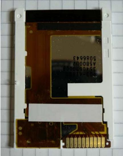
A photograph of an Epson L2F50 display assembly. It shows a white plastic frame with a black screen and a green circuit board at the bottom. A label on the screen reads "5086643" and "A58000". |
