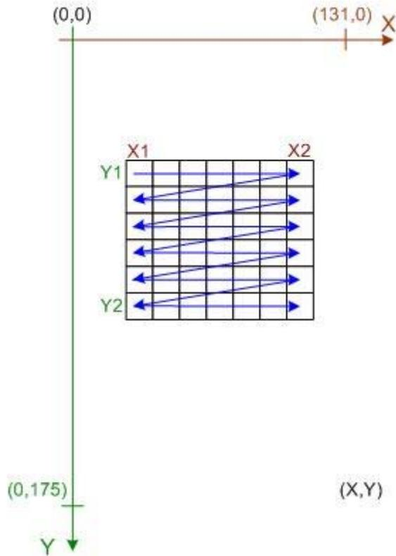
The display memory can be written in **X**- or **Y**-direction. Other advanced memory access modes are not supported. Writing in **Y**-direction is usually preferred if the display is used 90-degree rotated. If than the **X**- and **Y**-values in the PMEMWRY command are exchanged, the coordination system - shown in the left picture is obtained. In this case bitmaps are drawn from the upper left corner down to the lower right corner.
