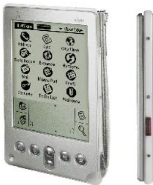
**Figure 2** The Handspring Visor Edge uses an IrDA port (red rectangle) to communicate with other PDAs and for synchronizing data with a PC.
