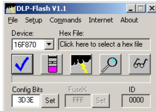
The application will search all connected USB devices attempting to locate one with a device description of “DLP-FLASH”. Once the programmer is located, the main program window will appear. If one is not found, an error message will be displayed.
