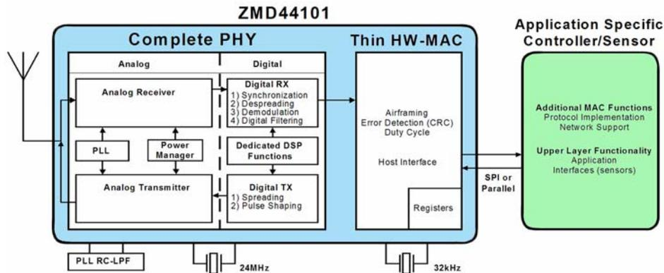
**Figure 2 – Sub-1 GHz Transceiver Block Diagram**
