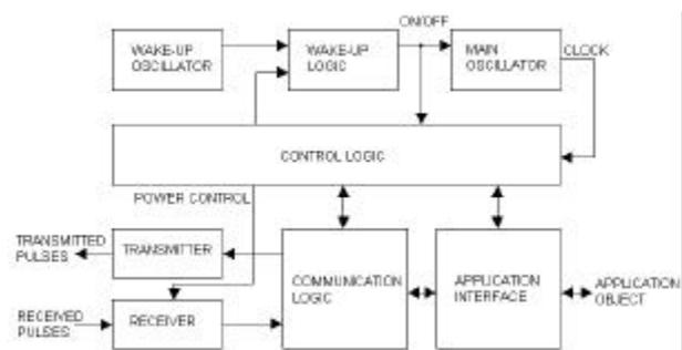
Figure 2: Functional block diagram of the TAG.
