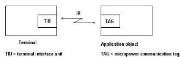
Figure 1: IR tag-based communication system.
