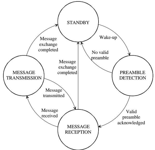
Figure 3: State diagram of the TAG communication logic.
