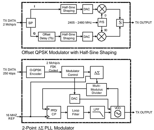
Figure 3. Transmitter Architectures.
