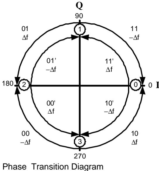
**Figure 1:** Symbol Set and Phase Transition Diagrams For ZigBee Modulation.
