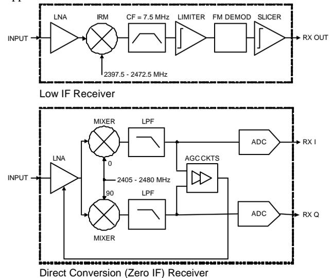
**Figure 2.** Receiver Architectures.
