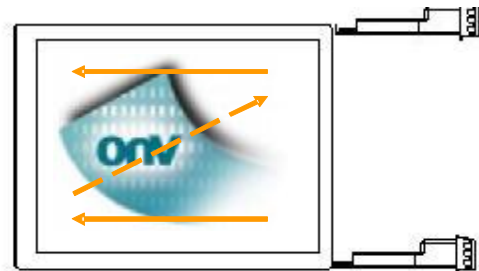
Fig. 2 Reverse scan (Pin19 = High)
