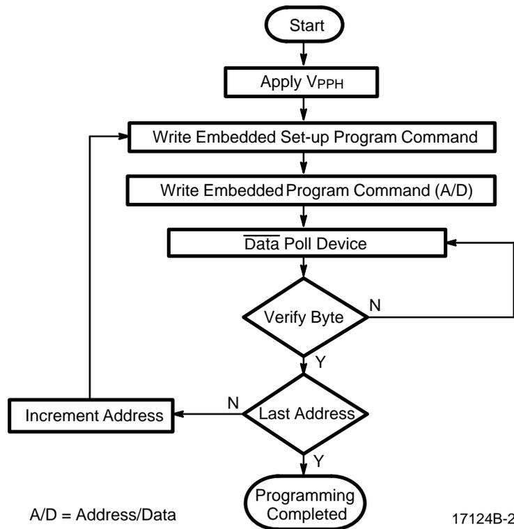
**Figure 2. Embedded Programming Algorithm**
