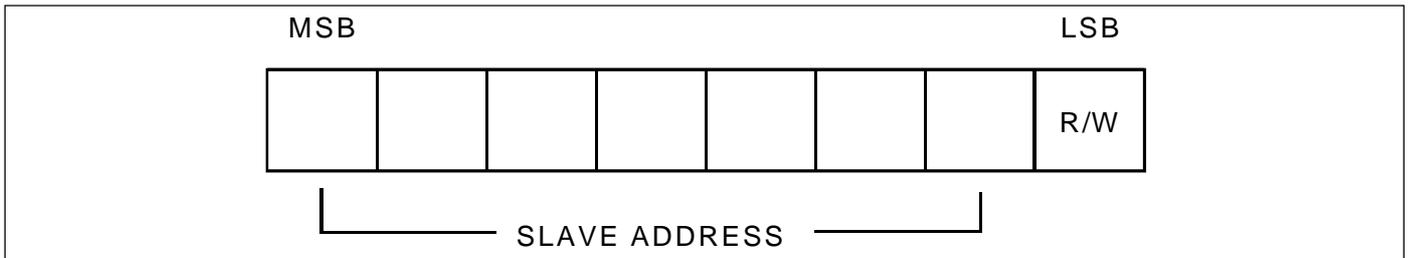
**Figure 4. First byte after the START condition**
