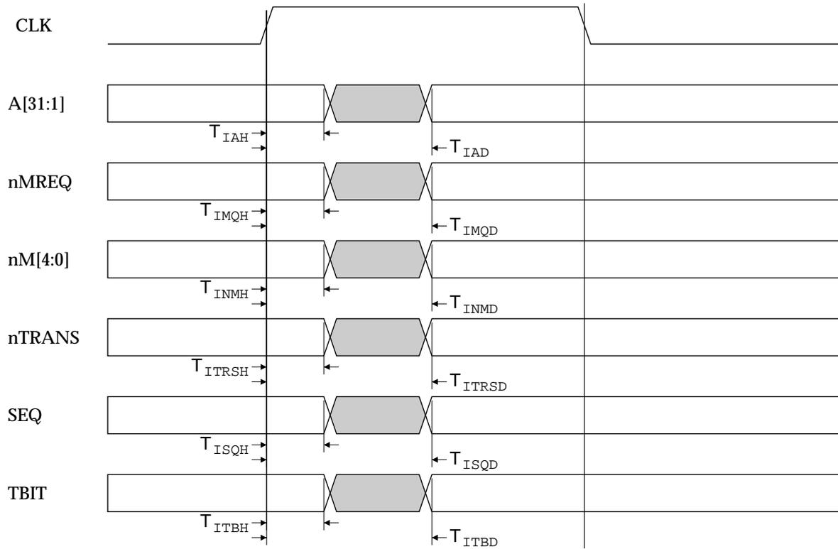
Figure 8-1 ARM9TDMI instruction memory interface output timing
