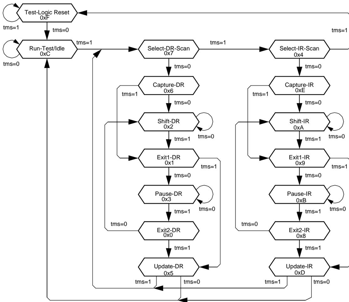
Figure 5-5 Test access port (TAP) controller state transitions
