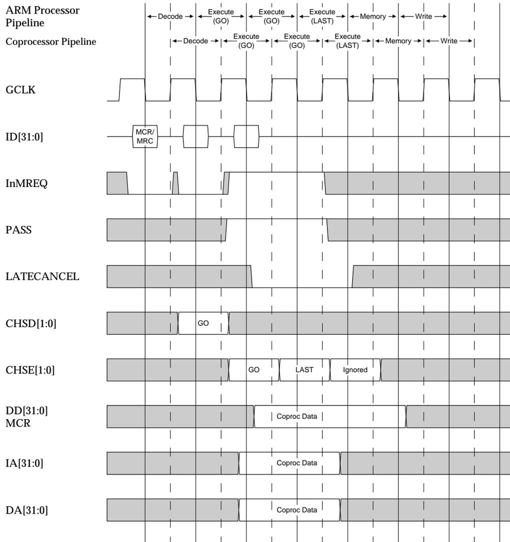
Figure 4-8 ARM9TDMI coprocessor 15 MCRs
