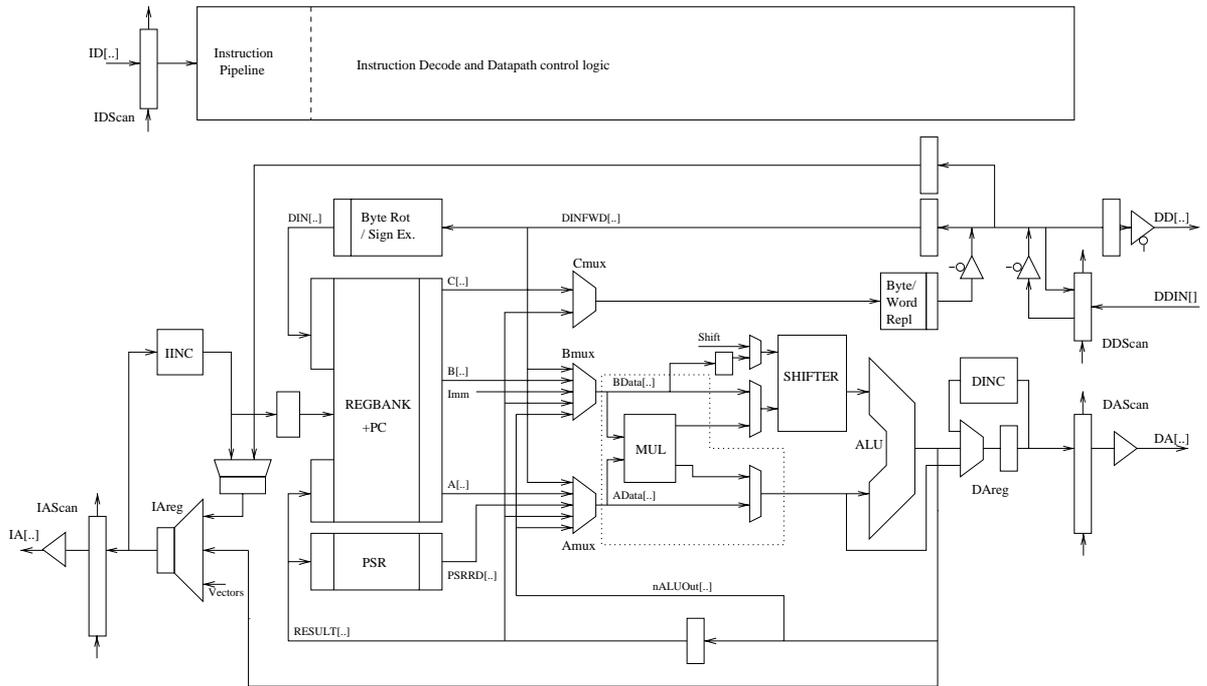
Figure 1-1 ARM9TDMI processor block diagram
