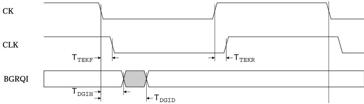
Figure 8-17 ARM9TDMI TCK related debug output timings
