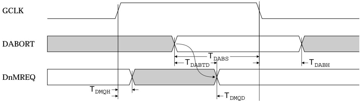
Figure 8-6 ARM9TDMI data ABORT and DnMREQ timing
