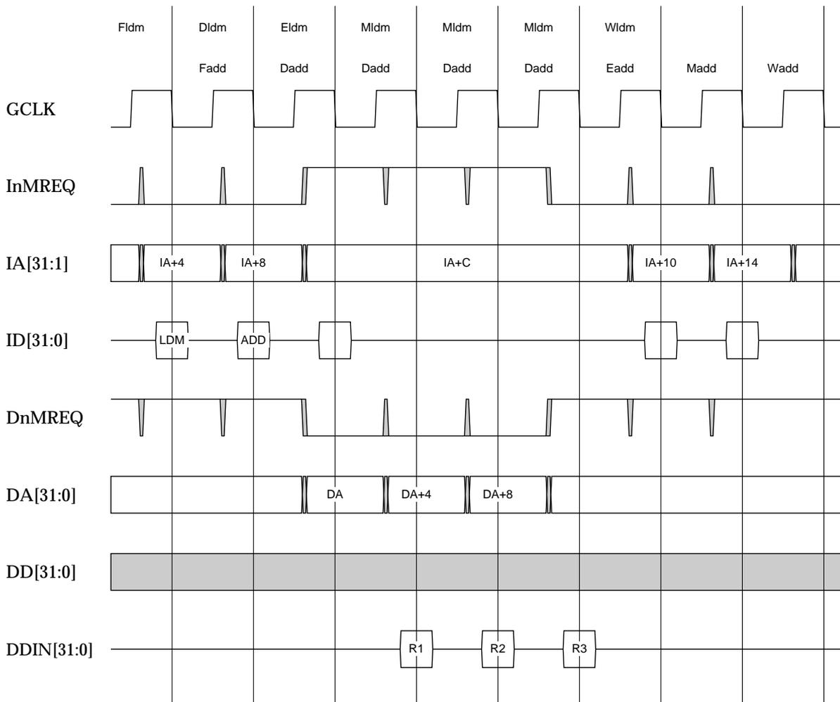
Figure 7-4 LDM dependent interlock
