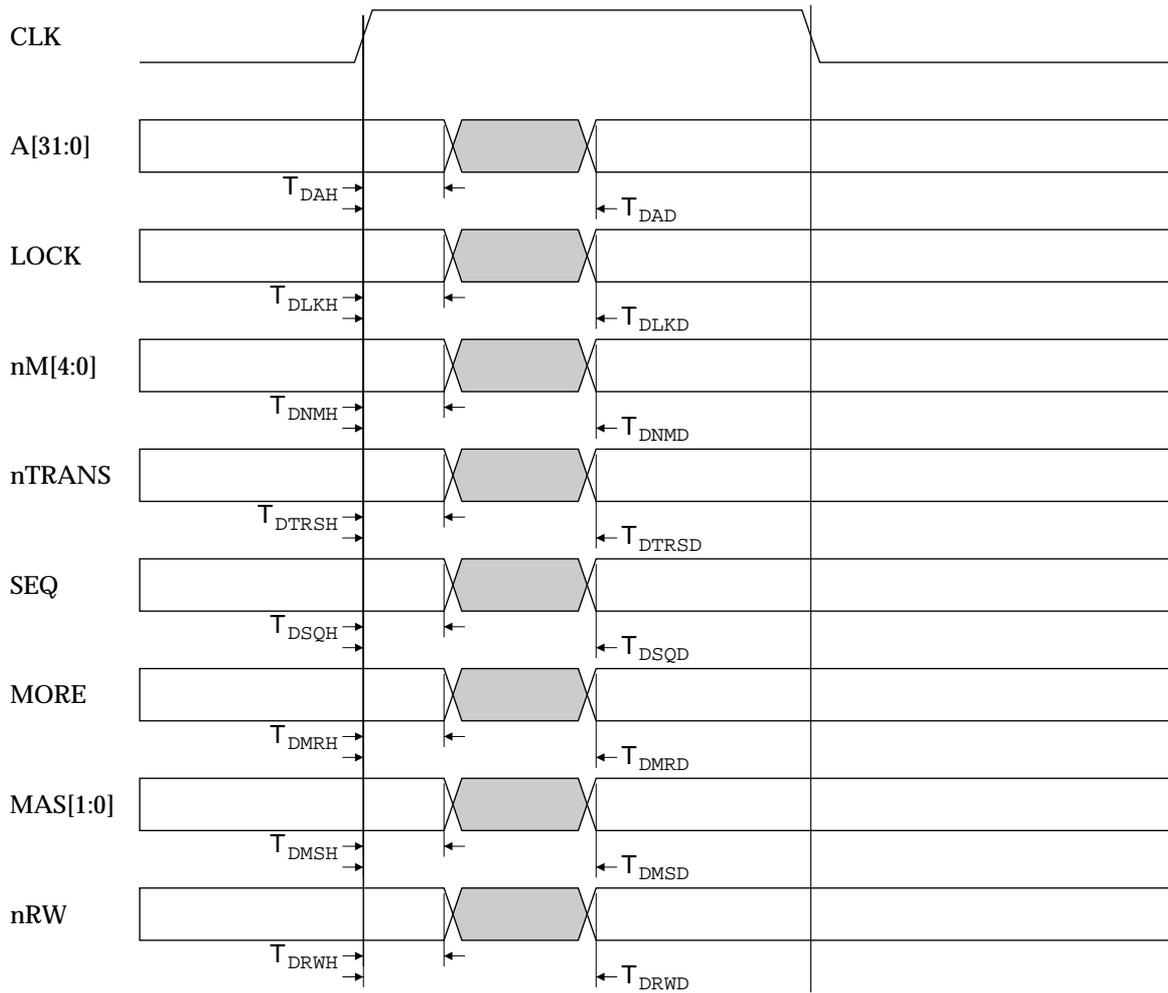
Figure 8-4 ARM9TDMI data memory interface output timing
