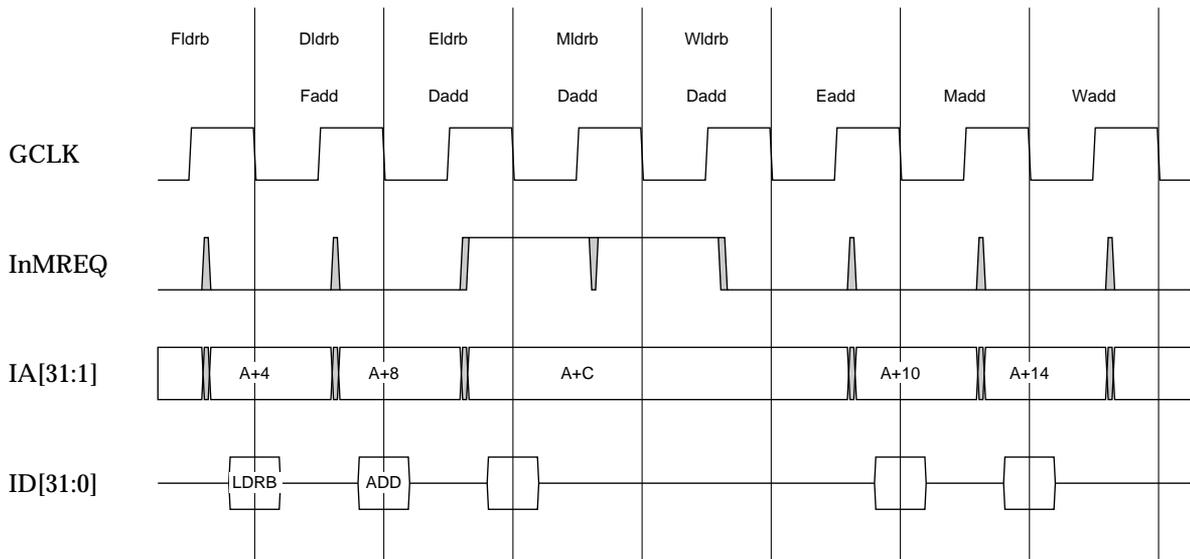
Figure 7-2 Two cycle load interlock
