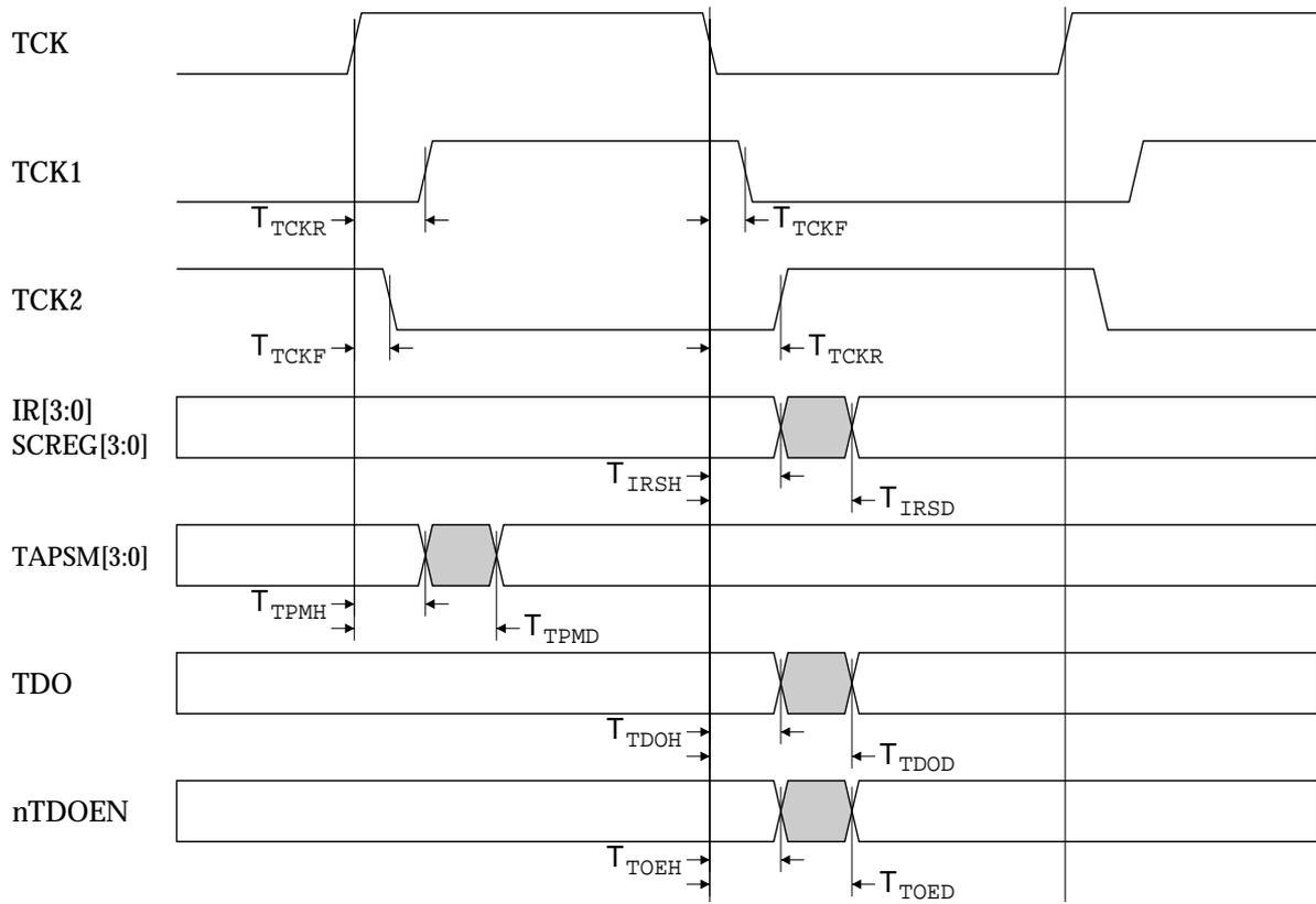
Figure 8-11 ARM9TDMI JTAG output signals
