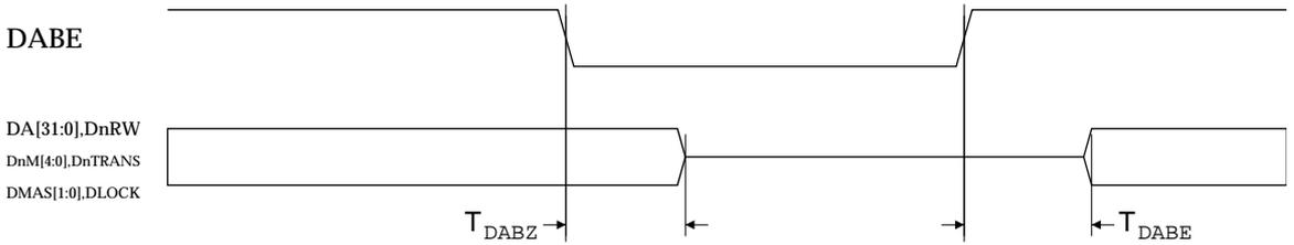
Figure 8-5 ARM9TDMI data address bus timing
