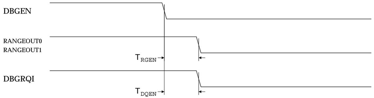
**Figure 8-20 ARM9TDMI DBGEN to output effects**
