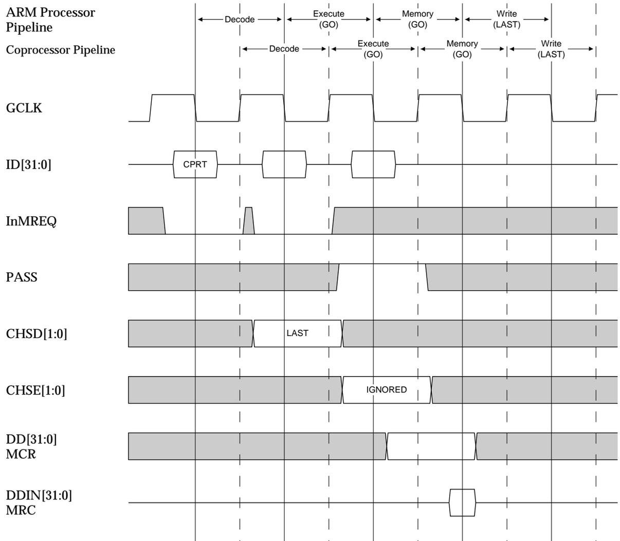
Figure 4-3 ARM9TDMI MCR / MRC transfer timing
