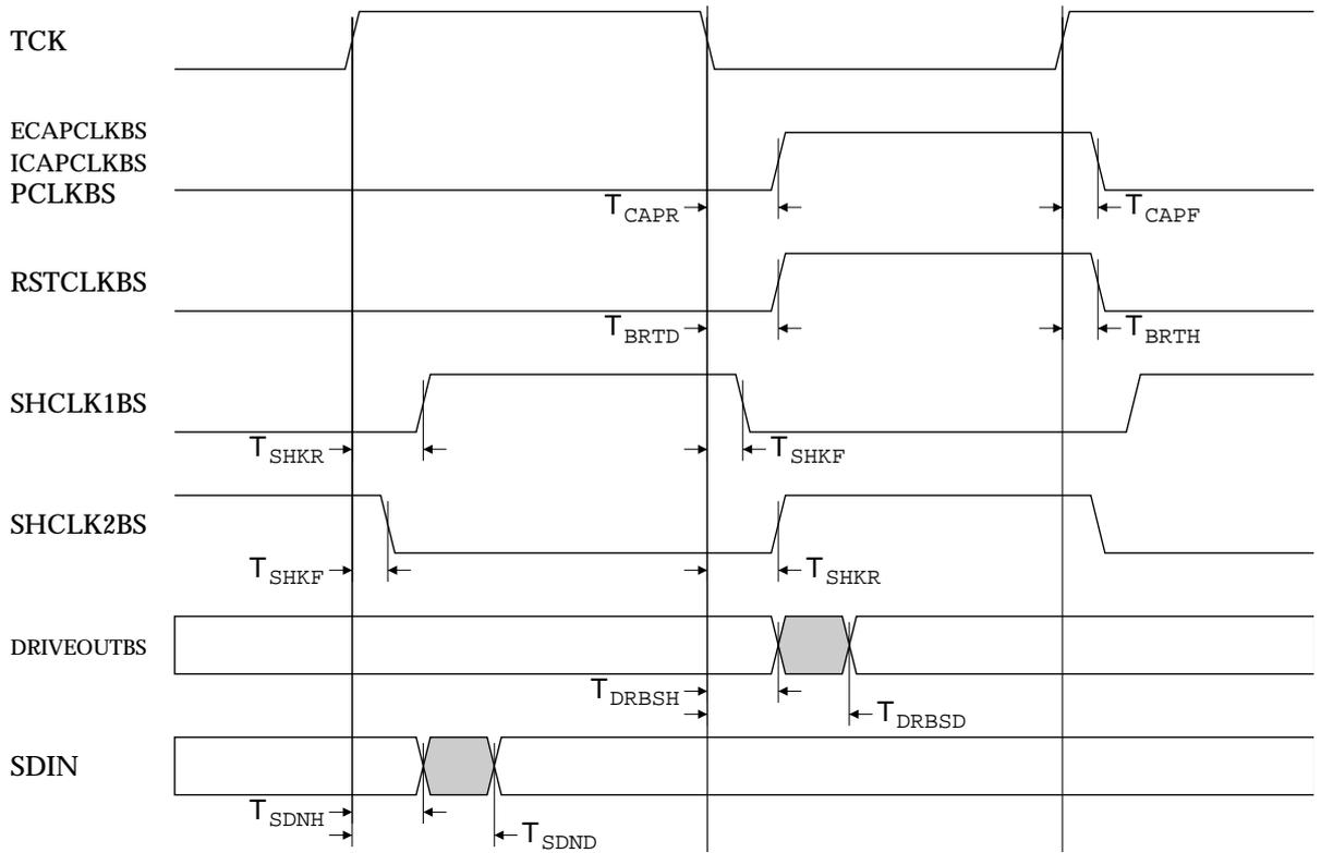
Figure 8-12 ARM9TDMI external boundary scan chain output signals
