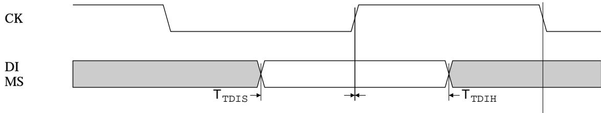
Figure 8-15 ARM9TDMI JTAG input signal timing
