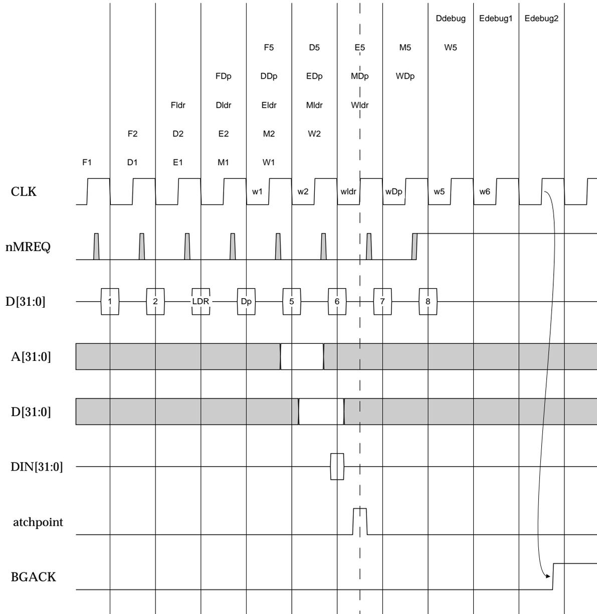
Figure 5-3 Watchpoint entry with data processing instruction
