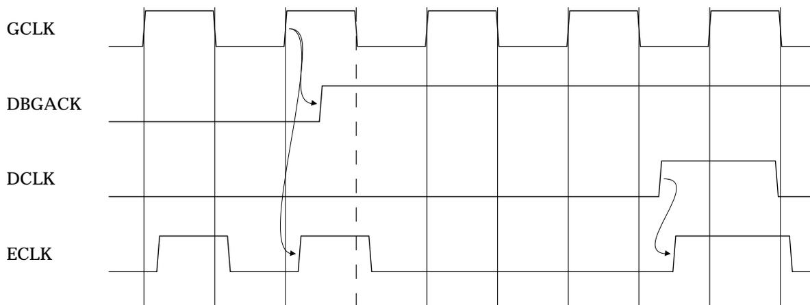
**Figure 5-6** Clock switching on entry to debug state
