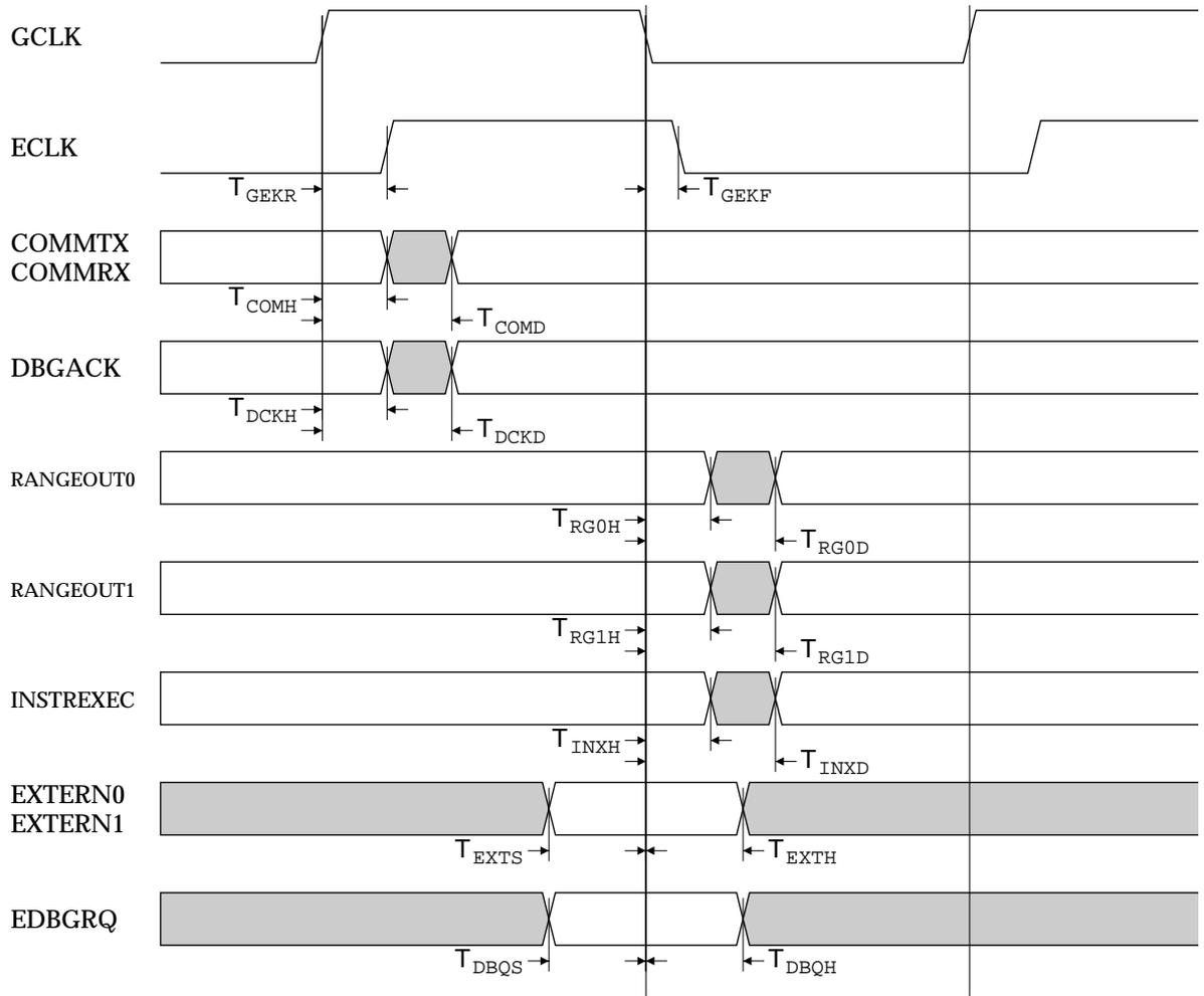
Figure 8-16 ARM9TDMI GCLK related debug output timings
