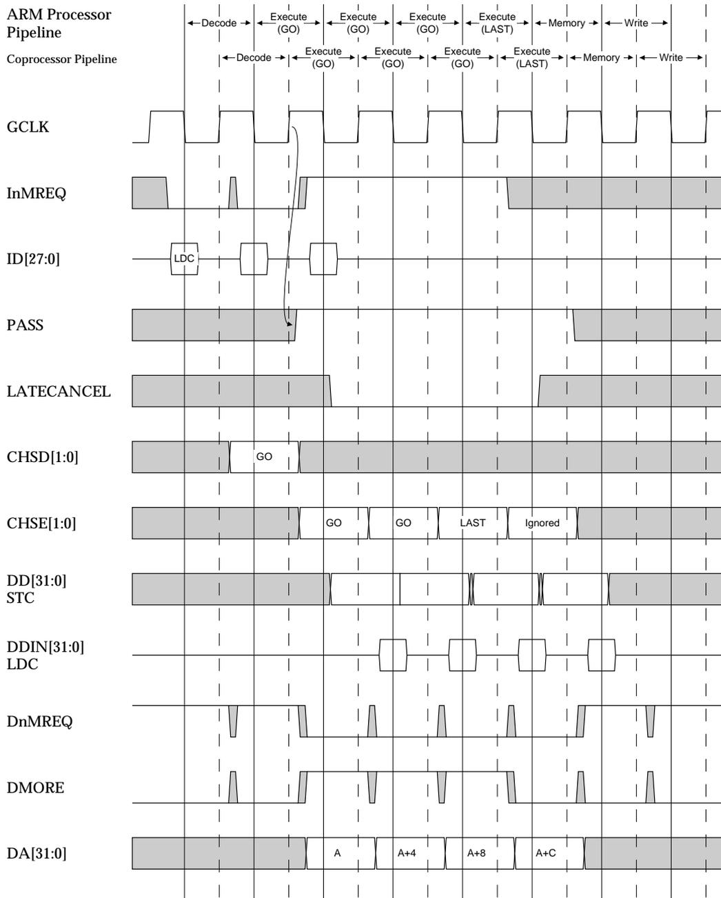
Figure 4-1 ARM9TDMI LDC / STC cycle timing
