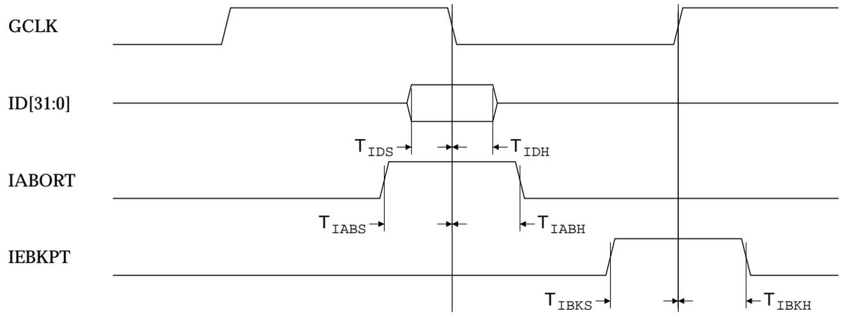
Figure 8-3 ARM9TDMI instruction memory interface input timing
