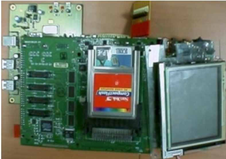
Figure 6. ISP1161 Evaluation, StrongBridge, StrongARM Development Kit and StrongARM Companion Chip Development Kit
