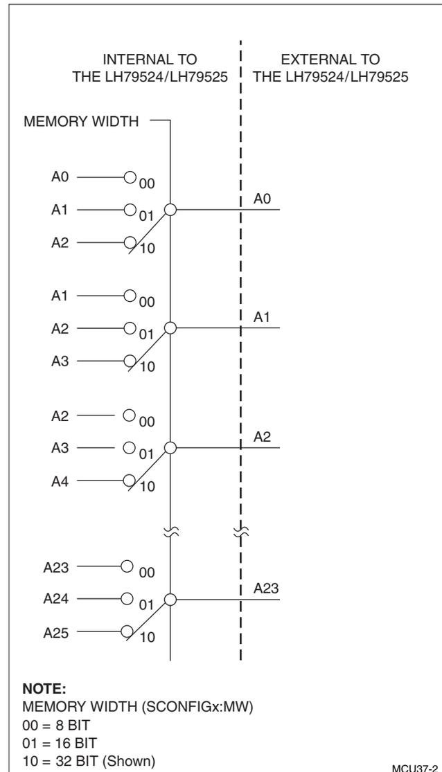
**Figure 1. Automatic Address Shifting**
