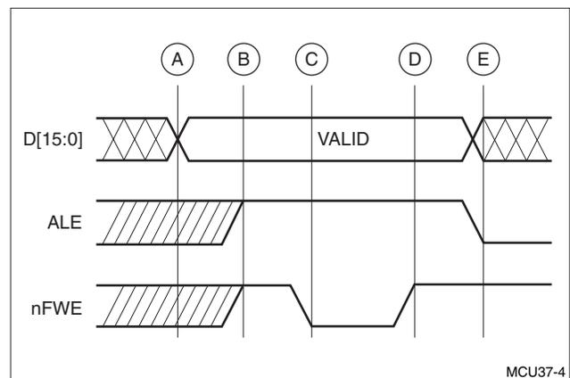
Figure 7. NAND Flash Timing Example
