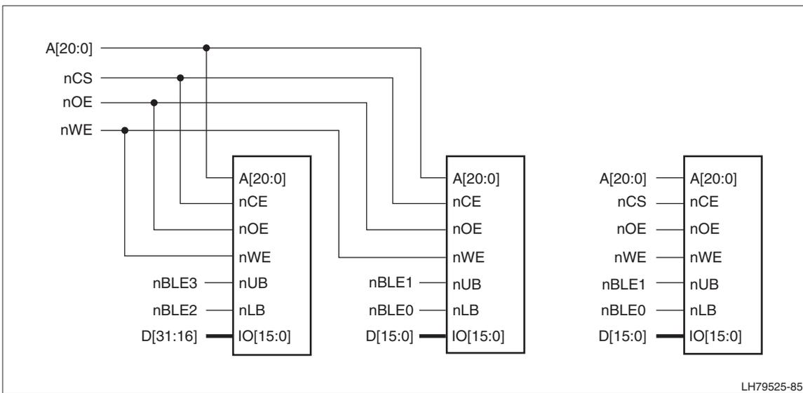
**Figure 3. Sixteen-bit Memory Connected for 32-bit System (left) and 16-bit System (right)**
