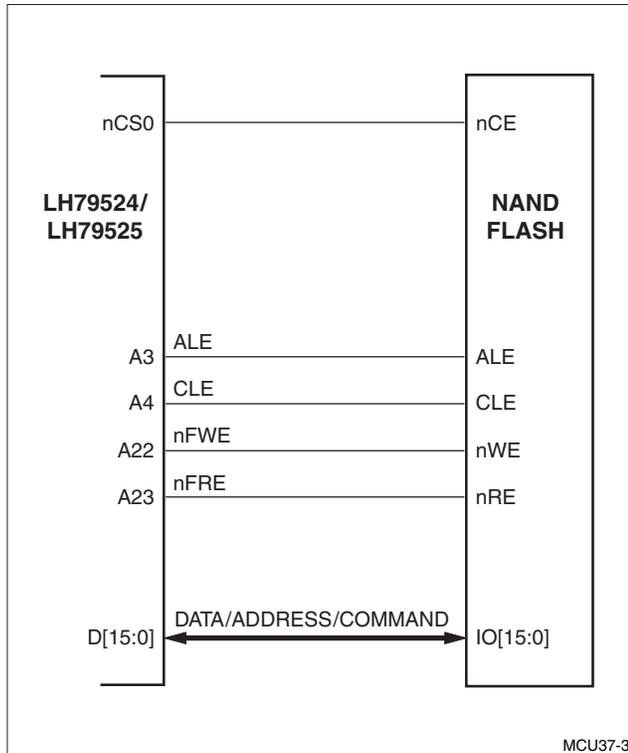
Figure 6. Connection to 16-bit NAND Flash
