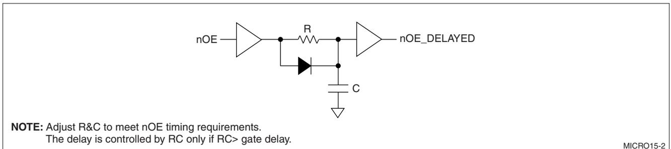
NOTE: Adjust R&C to meet nOE timing requirements. The delay is controlled by RC only if RC > gate delay.
