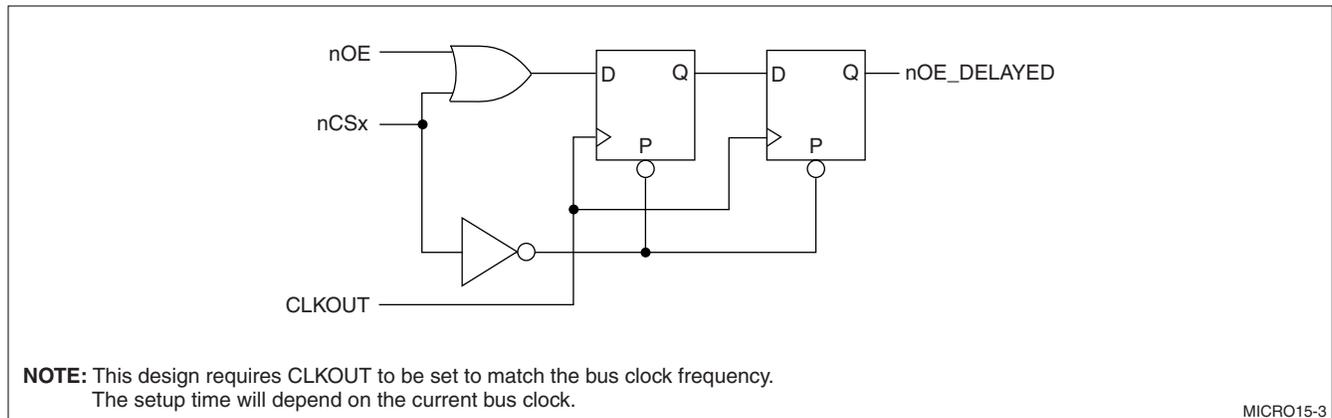
Figure 4. Delay Using Flip-flops
